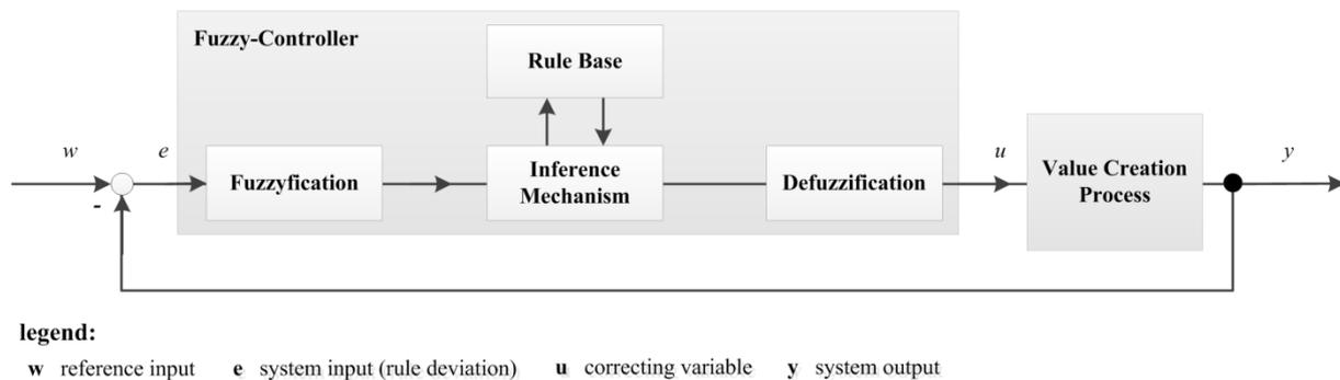
**FIG 5:** Schematic representation of a fuzzy controller
